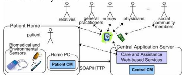
**Figure 6. Kamer Prototype System Architecture**
